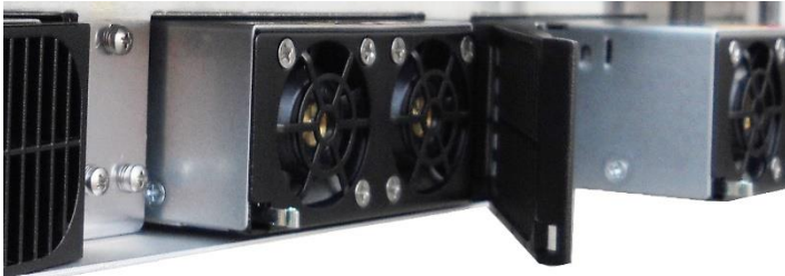
Detail of hot swappable power supply units on PFG NEXT
