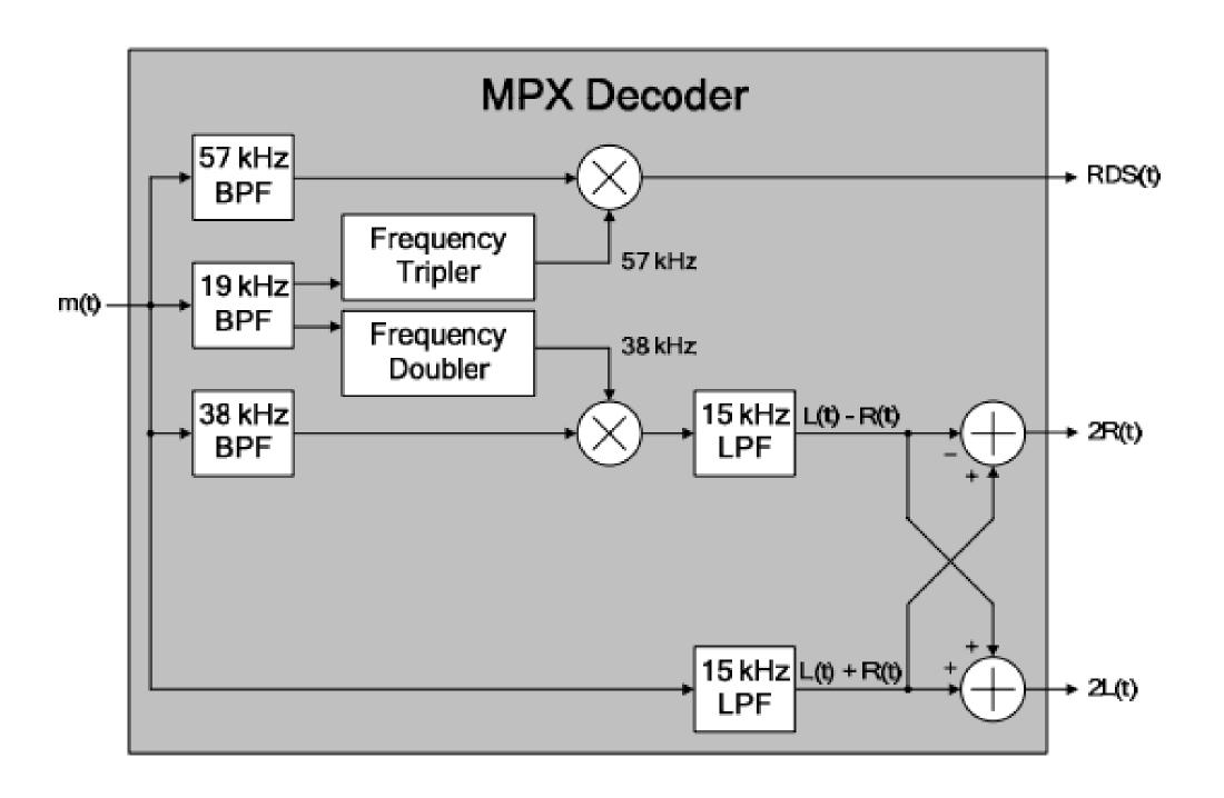
First the pilot tone at 19 kHz is doubled in frequency to 38 kHz. It is then fed into a mixer with the stereo difference signal to give the L - R signal at audio frequencies. Once the L + R and L - R signals are available they enter a matrix where they are added and subtracted to regenerate the L and R signals. At this point both signals are amplified separately in the normal way in a stereo amplifier before being converted into sound by loudspeakers or headphones.
