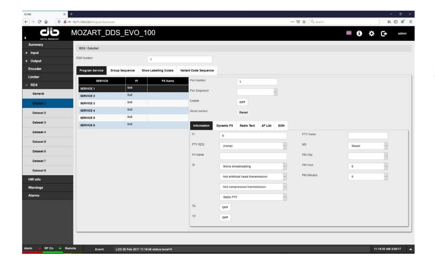
UECP messages are categorized into various groups including: RDS message commands, transparent data commands, paging commands, clock setting and control, RDS adjustment and control, control and set-up commands, bi-directional commands (i.e. remote configuration commands) and specific message commands. In the latter category, manufacturer specific commands are possible using a manufacturer ID, which can be obtained from the RDS Forum.
