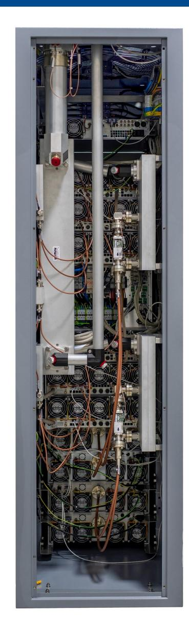
The PFG series of Modular FM transmitters is designed to operate in the whole 87.5 – 108 MHz frequency range for FM radio broadcasting applications and it covers a power range from 100W to 40kW.
