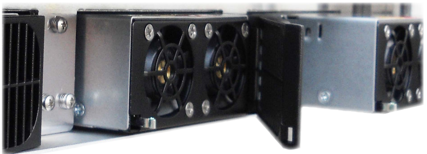
Detail of hot swappable power supply units on PFG NEXT
