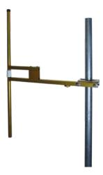
Wide band DAB dipole antennas in aluminum alodine. It is designed to work in one of the two sub-bands of DAB broadcast band (174 - 225 MHz or 200 - 240 MHz). The correct frequency must be specified at the moment of the order.
