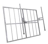
Wide band double dipole DAB antenna panels in stainless steel with PTFE insulator. It is designed to work in the whole DAB broadcast band (170 - 225 MHz).
