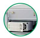
Hot-pluggable power supply units easily accessible from the front panel of amplifiers.
